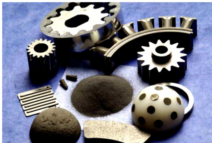
Figure (1): Examples of Powder metallurgy parts
