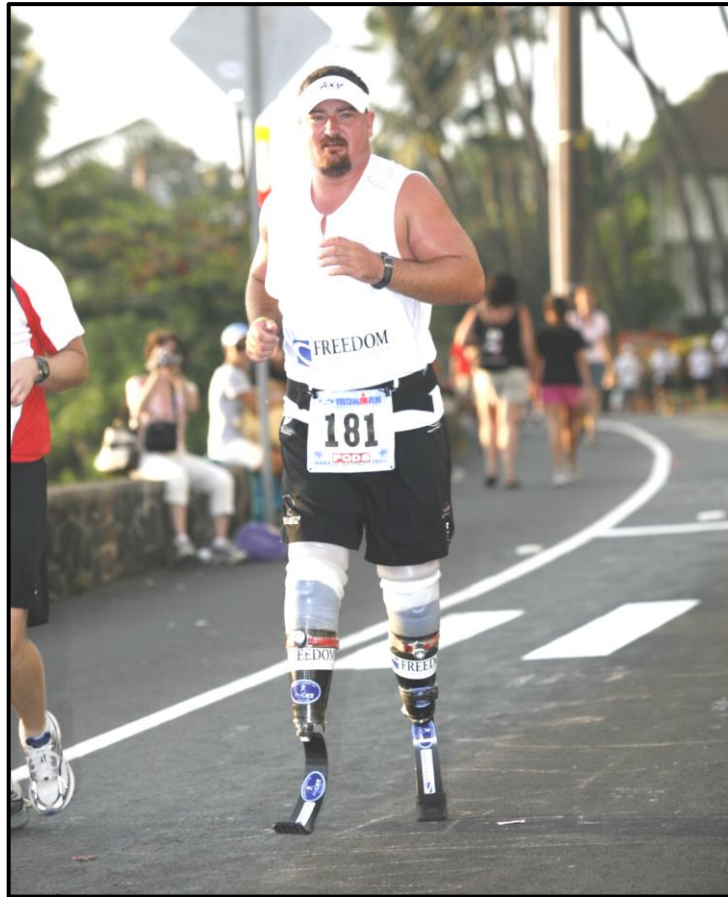
Figure 4. Running-specific foot modules are used to mimic natural running biomechanics.
