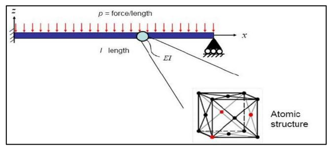
**Idea:** Consider the behavior of a collection of atoms inside the beam as deformation proceeds
