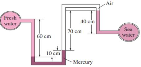
1035 kg/m<sup>3</sup>. Can the air column be ignored in the analysis?  $\rho_{air} = 1.2 \text{ kg/m}^3 \text{ b}$ ) replacing the air with oil whose specific gravity is 0.72. Ans. a) 3.39 kPa, b) 8.34 kPa.
