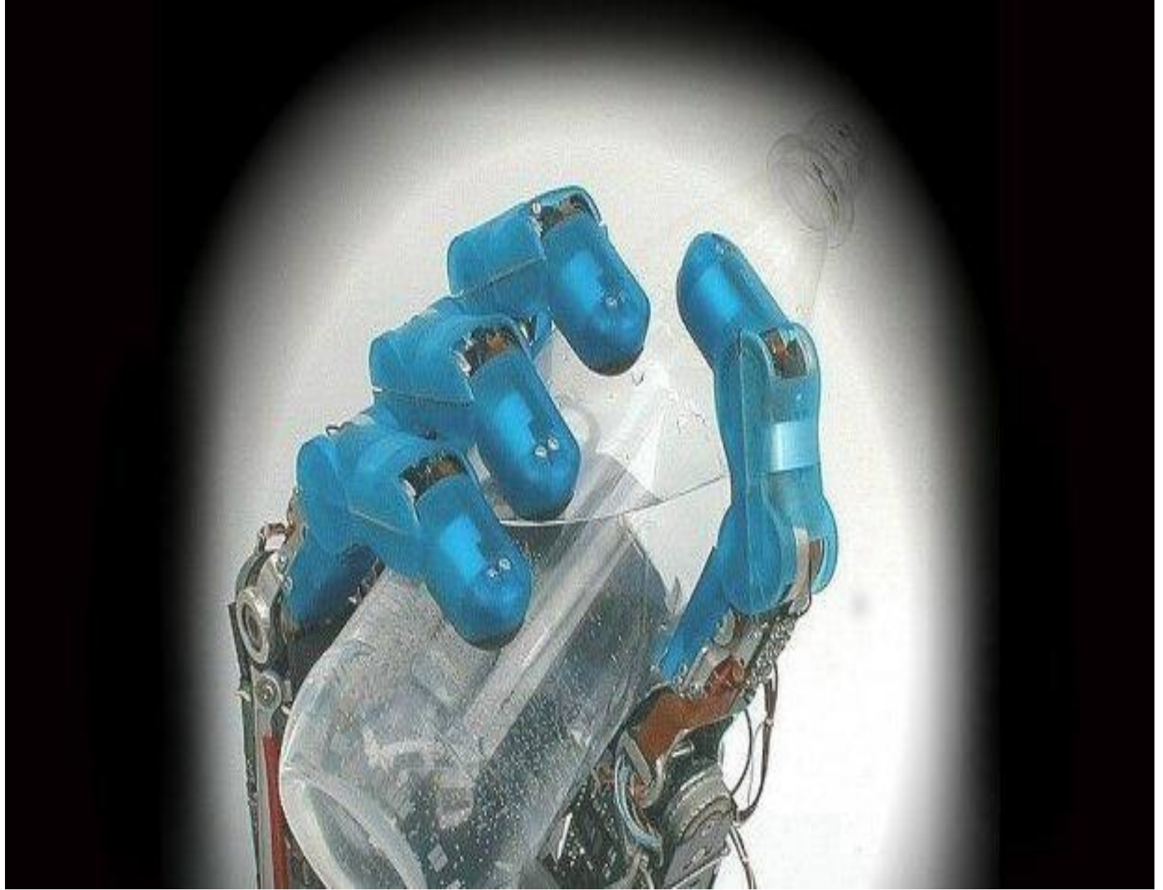
Robonaut flexible, five-fingered hand.
